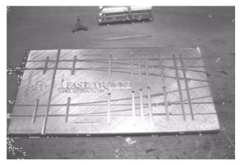
I'm convinced, though I haven't tried it, that these fixtures can also be used to build curved turnouts, by assembling them straight, then unsoldering a few ties from one rail, curving the rails, and resoldering the ties, also adjusting the point to stock rail fit
